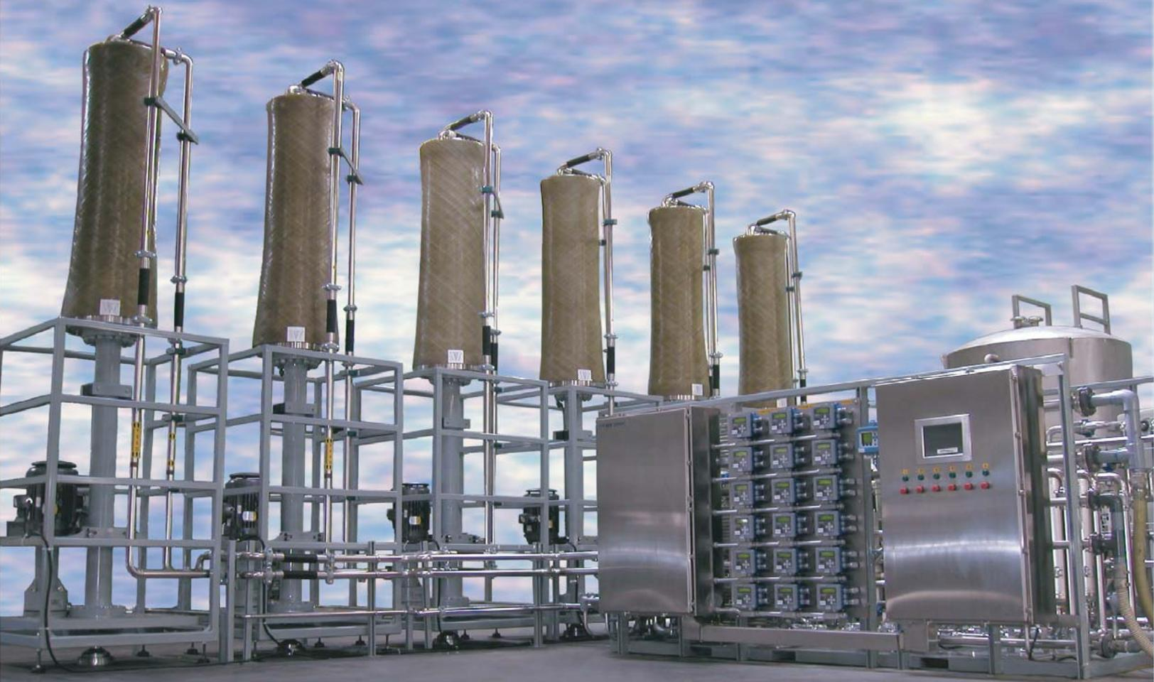
Vibrating Membrane Filtration System
