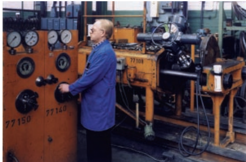
All valves are hydraulically tested up to pressures of 1164 barg.
