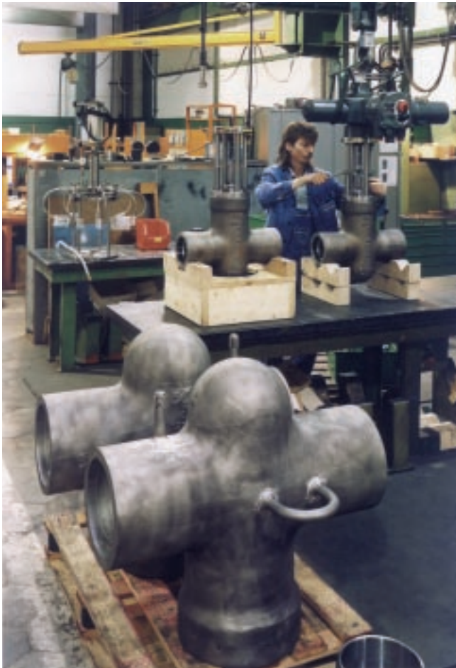
High pressure parallel slide valves in final assembly.
