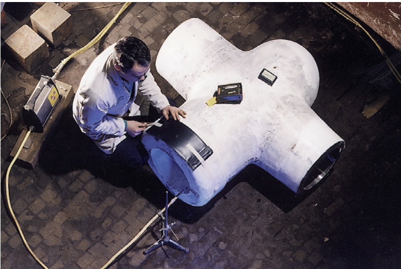
Radiographic and/or ultrasonic examination to ensure high integrity castings are provided.
