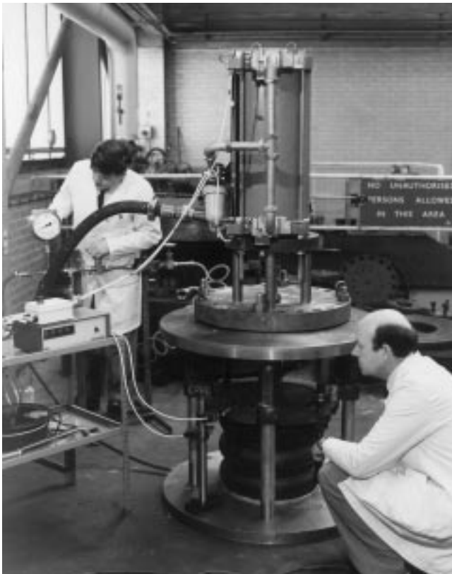
Pneumatic actuator functional test simulating increasing load over the full load.
