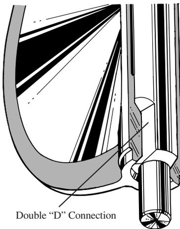
require difficult machining for disassembly. Disassembly of the Bray stem is just a matter of pulling the stem out of the disc. Without fasteners obstructing the line flow, the Series 30/31  $C_v$  values are higher than many other valves, turbulence is reduced, and pressure recovery is increased. The stem ends and top mounting flange are standardized for interchangeability with Bray actuators.
