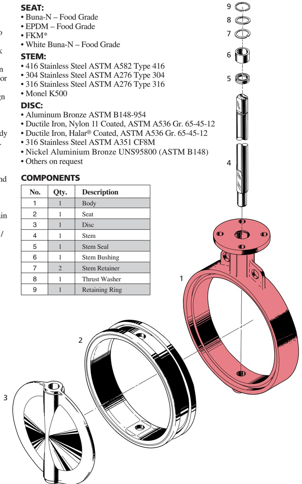
\*FKM is the ASTM D1418 designation for Fluorinated Hydrocarbon Elastomers (also called Fluoroelastomers).
