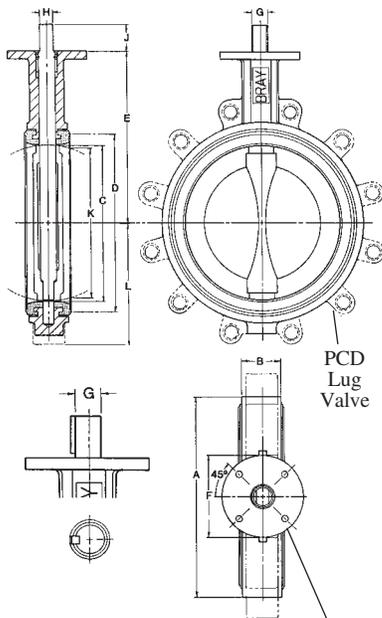
See chart for Actuator Mounting Flange Drilling.
