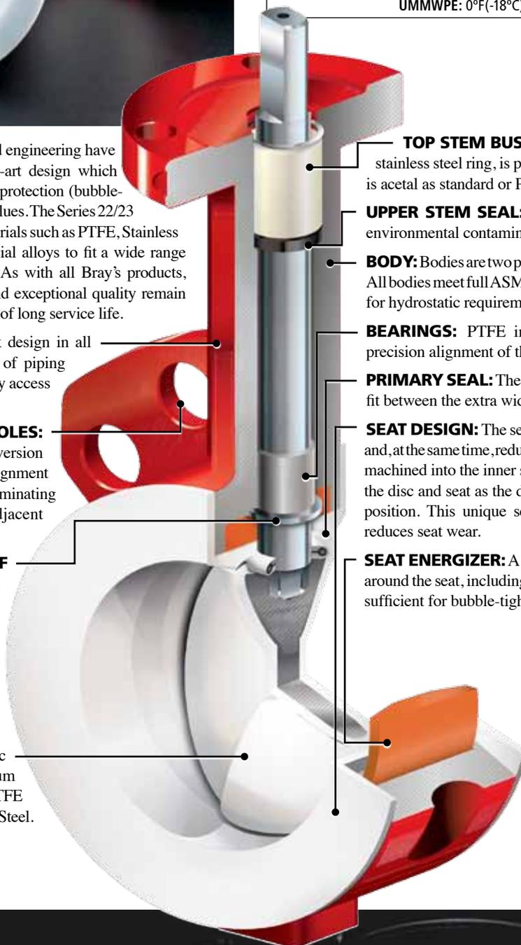
All Bray valves are pressure tested to 110% of rated pressure to assure bubble tight shutoff.
