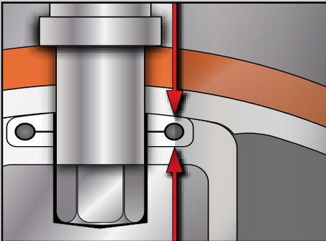
**BODY SEALS:** (Bidirectional): Reinforced PTFE gaskets are placed between the body halves. These seals eliminate contamination from external environmental conditions and potential leak path from the line media.
