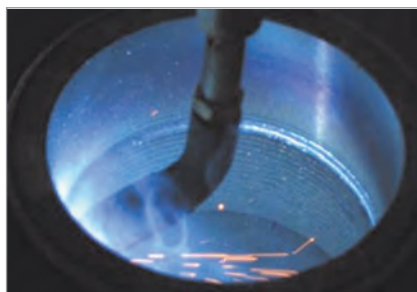
Weld Built Up
