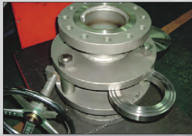
Step3. turn the spectacle plate 90 degree
