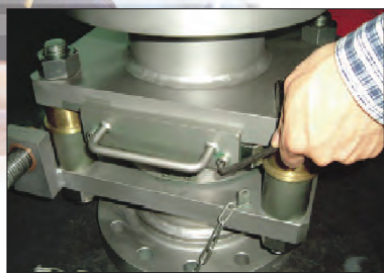
Step1. remove the end-plate of the blind
