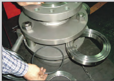
Step5. replace the internal O-ring
