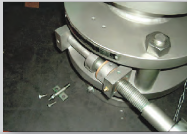
Step1. remove the position ass'y
