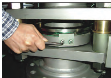
Step3. remove the both seat holder
