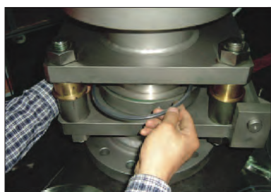
Step5. replace the internal O-ring
