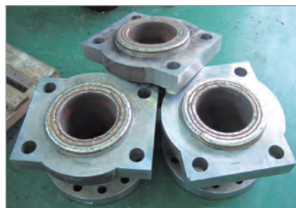
Weld Built Up
