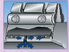
Fins on both ends of the gasket press on the pipe surface to create the seal.
