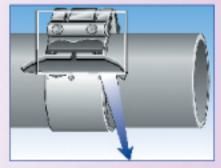
The hydraulic gasket, made of specially composed bacteriaresistant rubber, encloses the pipe and is covered with an external steel sheath.
