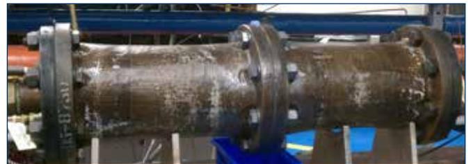
Style 3504 GYLON® STRESS SAVER® showed no signs of leakage when installed between smooth, flat face FRP flanges – the flange assembly was subjected to over 3,000 thermal cycles without a re-torque.
