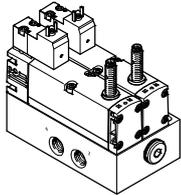
With the decentralised individual connection variant, the electrical connection for the control block is established as an individual connection to ISO 15407-1. The pneumatic connection is also established as an individual connection. With this variant, the two 5/2-way solenoid valves are pneumatically interlinked via two channels by means of the individual sub-base.
