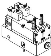
With the version of the control block for valve terminal VTSA/VTSA-F, the valves are actuated separately from the valve terminal via an individual electrical connection.
