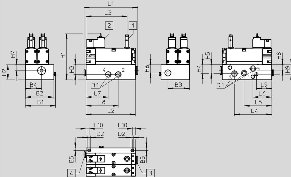
1 Proximity sensor PNP or NPN, size M8x1, plug connection to EN 61076-2-104
