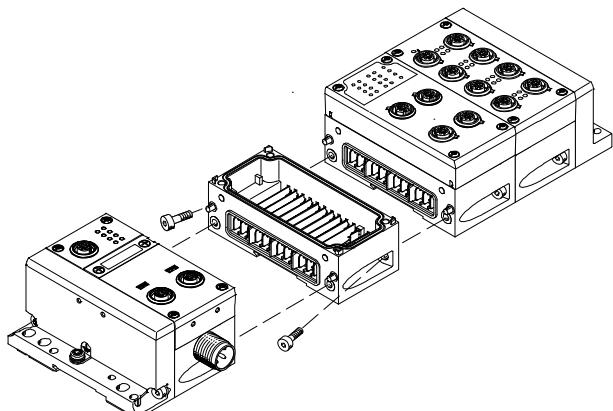
The CPX modules are mechanically connected using an angled fitting. The CPX terminal can thus be expanded at any time.
