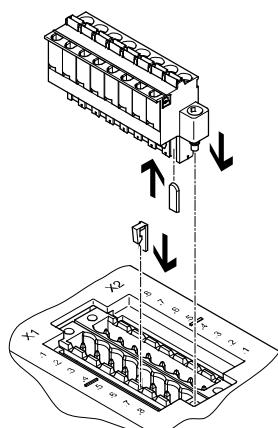
The connection block CPX-P-AB-2XKL-8POL and the sockets NECU-L3G8 can be matched to one another using the coding elements CPX-P-KDS-AB-2XKL.
