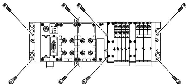
The end plates of the CPX terminal and valve terminal as well as the pneumatic interface include mounting holes for wall mounting. Additional mountings for the CPX terminal are available for longer valve terminals. These mountings differ depending on the design of the CPX terminal (polymer or metal).
