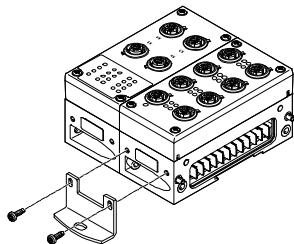
For longer valve terminals, there are additional mounting brackets for the CPX terminal that can be screwed onto the interlinking blocks. The mounting bracket CPX-M-BG-VT-2X enables a CPX terminal with valve terminal VTSA/VTSA-F/VTSA-F-CB to be mounted on a support system.
