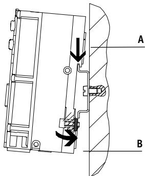
The H-rail mounting is part of the rear profile of the CPX interlinking blocks. The CPX terminal can be attached to the H-rail using the H-rail mounting kit. The CPX terminal is first hooked onto the H-rail (see arrow A).
