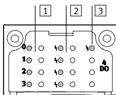
① Status LEDs for the inputs and outputs
