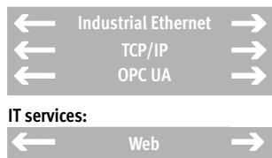
Gateway for continuous transfer of operating data from connected Festo components to a central storage location (cloud). Comprehensive status information for the gateway is displayed using 7 specific LEDs.
