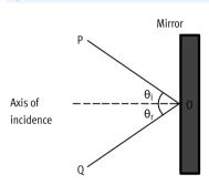
Specular reflection is the perfect reflection of light (or other kinds of wave) from a surface, when incident light from a single direction is reflected in a single direction.
