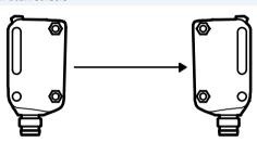
In the case of the through-beam sensor, the transmitter and receiver are located in different housings and must be installed opposite one another. Each object that interrupts the light beam between the transmitter and the receiver is detected. This is one of the most reliable principles in harsh environmental conditions. The disadvantage is that two separate components (transmitter and receiver) have to be wired and set up.
