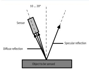
In the case of diffuse sensors with intensity differentiation, diffuse sensors with background suppression and distance and colour sensors, sensing is based on diffuse reflection. These sensors therefore require as much diffuse reflection as possible. Total reflection makes detection difficult and must therefore be avoided.
