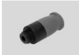
Plastic fitting for easy installation with one-hand operation. Hydrolysis resistant, FDA compliant and easy to clean. For pneumatic applications with a temperature range up to 60 °C and a pressure range up to 10 bar. Tubing outside diameter of 6 mm with connecting thread G $\frac{1}{8}$ .
