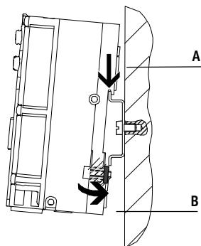
The H-rail mounting is part of the rear profile of the CPX-P interlinking blocks. The CPX-P terminal can be attached to the H-rail using the H-rail mounting kit. The CPX-P terminal is mounted on the H-rail (see arrow A) and
