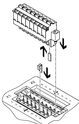
The connection blocks CPX-P-AB-2XKL-8POL and CPX-P-AB-2XKL-8POL-8DE-N-IS and the sockets NECU-L3G8 can be matched with one another using the coding elements CPX-P-KDS-AB-2XKL.
