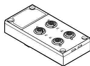
Direct machine mounting (connection block to IP65/IP67)
