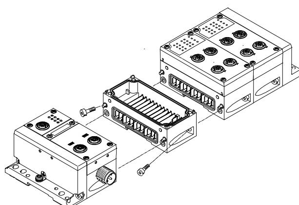
The mechanical connection between the CPX-P modules is created using angled screw connectors. The CPX-P terminal can thus be expanded at any time.
