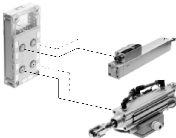
Support for the M12 connection block (8-pin) means that up to 4 cylinder-valve combinations with integrated sensors can be connected. Each cylinder-valve combination is supported by 2 inputs and 2 outputs per socket. It is therefore possible to control max. 2 solenoid coils and record signals from 2 sensors with a pre-assembled connecting cable.
