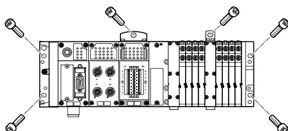
The end plates of the CPX-P terminal, the valve terminal and the pneumatic interface include mounting holes for wall mounting. Additional mountings for the CPX-P terminal are available for longer valve terminals.
