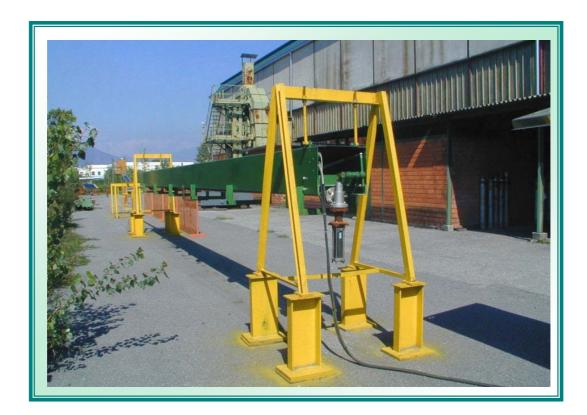
Testing for mechanical reliability of a longstroke retractable lance soot blower. The picture shows also the apparatus simulating steam pressure at valve inlet. Long lasting test have been carried out for different supports types and lubrificating devices.
