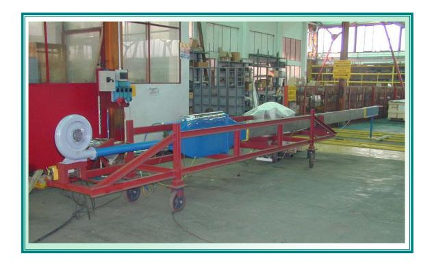
The above picture illustrates and equipment for heat transfer testing during calibration activities. The power is supplied by a set of electric resistances.
