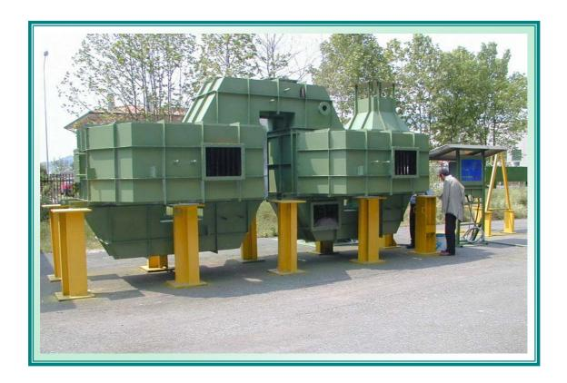
The above picture refers to a multipass heat exchangers realized by four horizontally settled modules.
