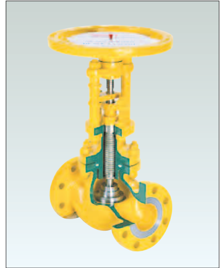
Bellows sealed globe valve Model 2100B. Bellows protected from the flow.
