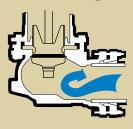
**Closed** — main valve held closed by operating nut and water pressure; barrel is dry.
