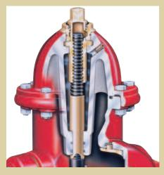
in the operating mechanism each time the hydrant is operated. Dual O-ring seals prevent lubricant loss during shipping, storage or installation and keep water away from stem threads and bearing surfaces when the hydrant is in use. An antifriction washer and automatic lubrication of the thrust collar add to easy operation.
