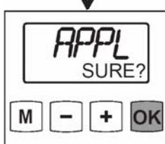
When changing application mode (VENT/HEAT). Push '+' and '-' keys at the same time 5 sec. This works with any display at top level.
