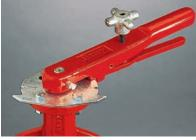
Infinite Position Notch Plate. for throttling applications, allows for very precise adjustments of valve disc positioning anywhere from 0° to 90°. Positioning is simply a matter of loosening the set knob, moving the handle, then retightening the knob. For resilient seated valves only.
