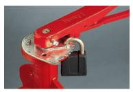
Padlock Kit allows the customer to lock the valve in the full open or closed position, tamper proofing the valve. By drilling a new hole in the top plate, the handle can be locked in mid travel.
