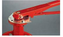
**Standard 10 Position Notch Plate** has been designed to lock the handle securely in place, preventing position change of disc due to line pressure, vibration or shock. Standard 8 Position Plate for high pressure valves is not shown.
