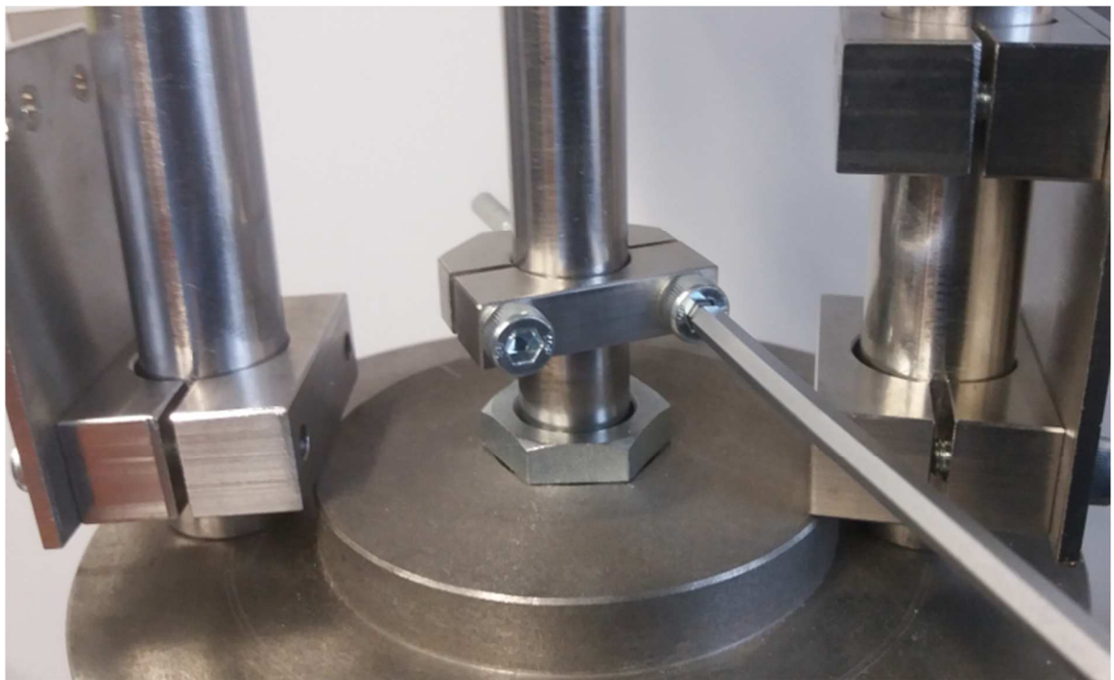
Fig. 84: Mounting valve clamp on the stem (elements are not tightened).
