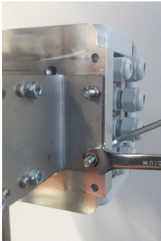
Fig. 88: Tightening positioner to the handles.
