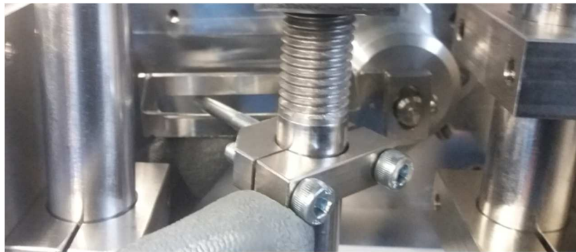
Fig. 90: Correct insertion of a screw coupling to the spring
