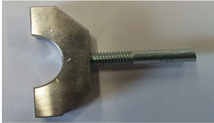
Fig. 81: Clamp of the stem with tightened screw.
