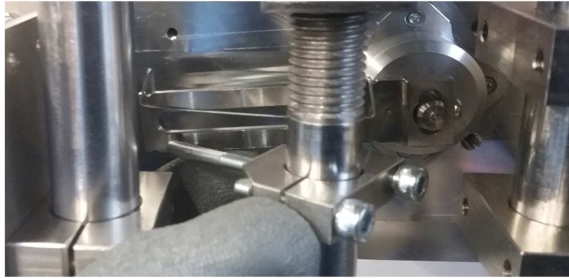
Fig. 89: Placing the coupling screw on the lever.
